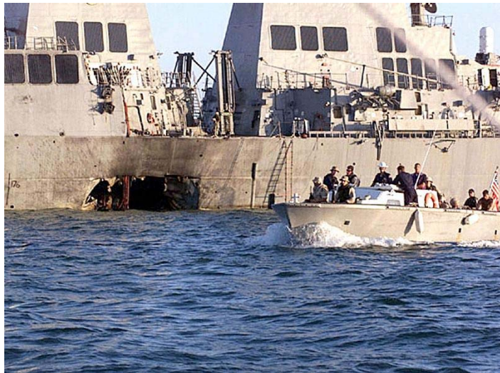
Figure 5-2. Suicide Bomb Damage to USS Cole . (Source: U.S. Navy)
